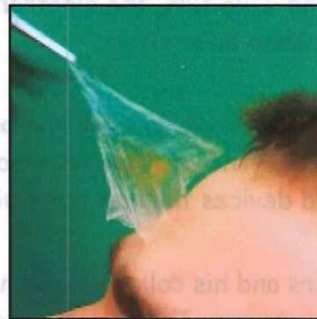
Stick like temporary tattoos. When attached to the head devices pick up electrical signals from the brain.
